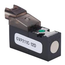
NITRA solenoid valve, 2-way, 2-position, N.C., single solenoid spring return, 10mm wide body, Cv=0.013, 12 VDC, miniature pin plug.
