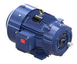
Marathon Globetrotter premium efficiency AC induction motor, general purpose, inverter rated and severe duty, 20hp, 3-phase, 230/460 VAC, 1800rpm, TEFC, NEMA 256TC frame, cast iron, C-face/rigid base mount.
