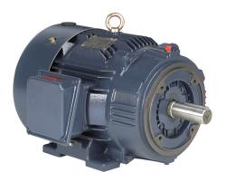
Marathon Globetrotter premium efficiency AC induction motor, general purpose, inverter rated and severe duty, 15hp, 3-phase, 230/460 VAC, 1800rpm, TEFC, NEMA 254TC frame, cast iron, C-face/rigid base mount.
