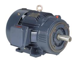
Marathon Globetrotter premium efficiency AC induction motor, general purpose, inverter rated and hazardous location, 15hp, 3-phase, 230/460 VAC, 1800rpm, TEFC, 254TC frame, cast iron, C-face/rigid base mount.
