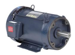
Marathon Globetrotter premium efficiency AC induction motor, general purpose and inverter rated, 10hp, 3-phase, 230/460 VAC, 1800rpm, TEFC, NEMA 215TC frame, rolled steel, C-face/rigid base mount.
