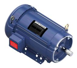
Marathon Globetrotter premium efficiency AC induction motor, general purpose and inverter rated, 7-1/2hp, 3-phase, 230/460 VAC, 1800rpm, TEFC, NEMA 213TC frame, rolled steel, Cface/rigid base mount.
