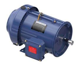
Marathon Globetrotter premium efficiency AC induction motor, general purpose and inverter rated, 5hp, 3-phase, 230/460 VAC, 1800rpm, TEFC, NEMA 184TC frame, rolled steel, C-face/rigid base mount.
