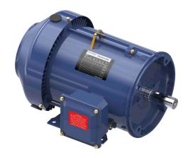
Marathon Globetrotter premium efficiency AC induction motor, general purpose and inverter rated, 5hp, 3-phase, 230/460 VAC, 3600rpm, TEFC, NEMA 184TC frame, rolled steel, C-face/rigid base mount.
