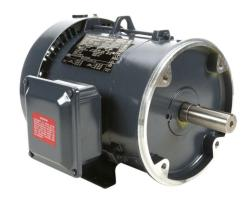
Marathon Globetrotter premium efficiency AC induction motor, general purpose and inverter rated, 3hp, 3-phase, 230/460 VAC, 1800rpm, TEFC, NEMA 182TC frame, rolled steel, C-face/rigid base mount.
