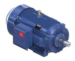
Marathon Globetrotter premium efficiency AC induction motor, general purpose, inverter rated and severe duty, 200hp, 3-phase, 460 VAC, 1800rpm, TEFC, 447T frame, cast iron, rigid base mount.
