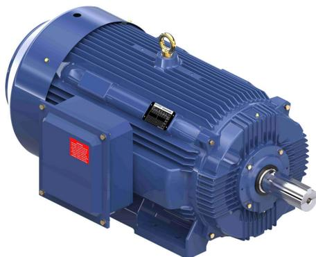
Marathon Globetrotter premium efficiency AC induction motor, general purpose, inverter rated and severe duty, 200hp, 3-phase, 460 VAC, 1800rpm, TEFC, NEMA 447T frame, cast iron, rigid base mount.
