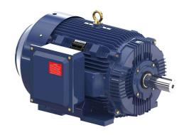
Marathon Globetrotter premium efficiency AC induction motor, general purpose, inverter rated and severe duty, 150hp, 3-phase, 460 VAC, 1800rpm, TEFC, NEMA 445T frame, cast iron, rigid base mount.
