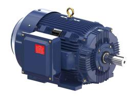
Marathon Globetrotter premium efficiency AC induction motor, general purpose, inverter rated and severe duty, 150hp, 3-phase, 460 VAC, 1800rpm, TEFC, 445T frame, cast iron, rigid base mount.
