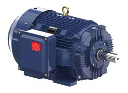
Marathon Globetrotter premium efficiency AC induction motor, general purpose, inverter rated and severe duty, 125hp, 3-phase, 460 VAC, 1800rpm, TEFC, NEMA 444T frame, cast iron, rigid base mount.
