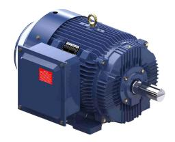
Marathon Globetrotter premium efficiency AC induction motor, general purpose, inverter rated and severe duty, 100hp, 3-phase, 230/460 VAC, 1800rpm, TEFC, NEMA 405T frame, cast iron, rigid base mount.
