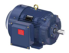
Marathon Globetrotter premium efficiency AC induction motor, general purpose, inverter rated and severe duty, 75hp, 3-phase, 230/460 VAC, 1800rpm, TEFC, 365T frame, cast iron, rigid base mount.
