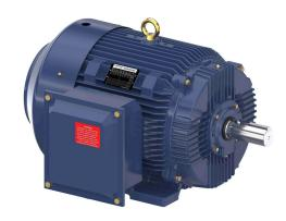
Marathon Globetrotter premium efficiency AC induction motor, general purpose, inverter rated and severe duty, 75hp, 3-phase, 230/460 VAC, 1800rpm, TEFC, NEMA 365T frame, cast iron, rigid base mount.
