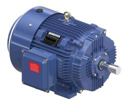
Marathon Globetrotter premium efficiency AC induction motor, general purpose, inverter rated and severe duty, 50hp, 3-phase, 230/460 VAC, 1800rpm, TEFC, NEMA 326T frame, cast iron, rigid base mount.
