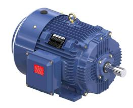
Marathon Globetrotter premium efficiency AC induction motor, general purpose, inverter rated and severe duty, 40hp, 3-phase, 230/460 VAC, 1800rpm, TEFC, 324T frame, cast iron, rigid base mount.
