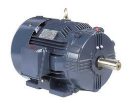
Marathon Globetrotter premium efficiency AC induction motor, general purpose, inverter rated and severe duty, 30hp, 3-phase, 208-230/460 VAC, 1800rpm, TEFC, 286T frame, cast iron, rigid base mount.
