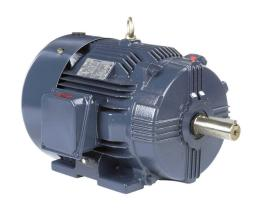
Marathon Globetrotter premium efficiency AC induction motor, general purpose, inverter rated and severe duty, 30hp, 3-phase, 208-230/460 VAC, 1800rpm, TEFC, NEMA 286T frame, cast iron, rigid base mount.
