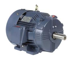
Marathon Globetrotter premium efficiency AC induction motor, general purpose, inverter rated and severe duty, 25hp, 3-phase, 208-230/460 VAC, 1800rpm, TEFC, NEMA 284T frame, cast iron, rigid base mount.
