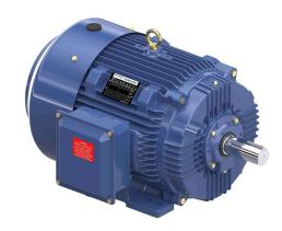
Marathon Globetrotter premium efficiency AC induction motor, general purpose, inverter rated and severe duty, 20hp, 3-phase, 208-230/460 VAC, 1800rpm, TEFC, 256T frame, cast iron, rigid base mount.
