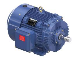
Marathon Globetrotter premium efficiency AC induction motor, general purpose, inverter rated and severe duty, 20hp, 3-phase, 208-230/460 VAC, 1800rpm, TEFC, NEMA 256T frame, cast iron, rigid base mount.
