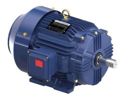
Marathon Globetrotter premium efficiency AC induction motor, general purpose, inverter rated and severe duty, 10hp, 3-phase, 208-230/460 VAC, 1800rpm, TEFC, NEMA 215T frame, cast iron, rigid base mount.
