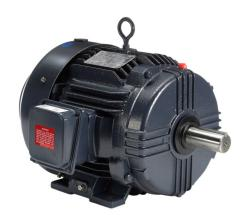
Marathon Globetrotter premium efficiency AC induction motor, general purpose, inverter rated and hazardous location, 7-1/2hp, 3-phase, 208-230/460 VAC, 1800rpm, TEFC, 213T frame, cast iron, rigid base mount.
