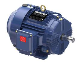
Marathon Globetrotter premium efficiency AC induction motor, general purpose, inverter rated and severe duty, 5hp, 3-phase, 208-230/460 VAC, 1800rpm, TEFC, NEMA 184T frame, cast iron, rigid base mount.
