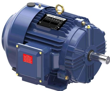
Marathon Globetrotter premium efficiency AC induction motor, general purpose, inverter rated and severe duty, 3hp, 3-phase, 208-230/460 VAC, 1800rpm, TEFC, NEMA 182T frame, cast iron, rigid base mount.
