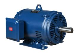
Marathon Globetrotter premium efficiency AC induction motor, general purpose and inverter rated, 50hp, 3-phase, 208-230/460 VAC, 1800rpm, ODP, NEMA 326T frame, rolled steel, rigid base mount.
