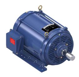
Marathon Globetrotter premium efficiency AC induction motor, general purpose and inverter rated, 30hp, 3-phase, 208-230/460 VAC, 1800rpm, ODP, NEMA 286T frame, rolled steel, rigid base mount.
