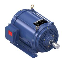
Marathon Globetrotter premium efficiency AC induction motor, general purpose and inverter rated, 25hp, 3-phase, 208-230/460 VAC, 1800rpm, ODP, NEMA 284T frame, rolled steel, rigid base mount.
