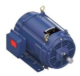
Marathon Globetrotter premium efficiency AC induction motor, general purpose and inverter rated, 15hp, 3-phase, 208-230/460 VAC, 1800rpm, ODP, 254T frame, rolled steel, rigid base mount.
