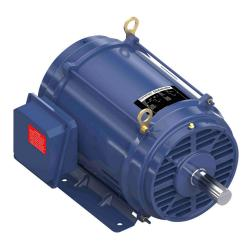
Marathon Globetrotter premium efficiency AC induction motor, general purpose and inverter rated, 15hp, 3-phase, 208-230/460 VAC, 1800rpm, ODP, NEMA 254T frame, rolled steel, rigid base mount.
