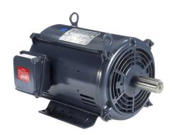
Marathon Globetrotter premium efficiency AC induction motor, general purpose and inverter rated, 10hp, 3-phase, 208-230/460 VAC, 1800rpm, ODP, 215T frame, rolled steel, rigid base mount.
