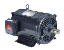
Marathon Globetrotter premium efficiency AC induction motor, general purpose and inverter rated, 10hp, 3-phase, 208-230/460 VAC, 1800rpm, ODP, NEMA 215T frame, rolled steel, rigid base mount.
