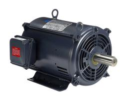
Marathon Globetrotter premium efficiency AC induction motor, general purpose and inverter rated, 7-1/2hp, 3-phase, 208-230/460 VAC, 1800rpm, ODP, NEMA 213T frame, rolled steel, rigid base mount.
