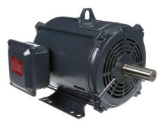
Marathon Globetrotter premium efficiency AC induction motor, general purpose and inverter rated, 5hp, 3-phase, 208-230/460 VAC, 1800rpm, ODP, NEMA 184T frame, rolled steel, rigid base mount.
