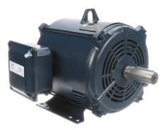
Marathon Globetrotter premium efficiency AC induction motor, general purpose and inverter rated, 3hp, 3-phase, 208-230/460 VAC, 1800rpm, ODP, NEMA 182T frame, rolled steel, rigid base mount.
