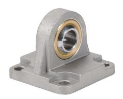
NITRA rear spherical pivot, spherical bearing, zinc plated steel. For use with 40mm bore G-series cylinders.
