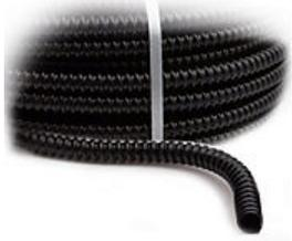
Iboco I-Flex flexible electrical tubing, liquid-tight, PVC, 3/8in trade size, black, 98ft/29.8m coil length.
