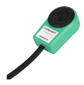
IronHorse encoder, 5-24 VDC, NPN open collector output, 1/10/20 ppr, 61mm diameter body, NEMA 3R, IP14, 6ft cable length, pigtail. For use with GSD8 series DC drives. Mounting hardware and (3) magnets included.
