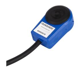
IronHorse encoder, 5-24 VDC, NPN open collector output, 1/10/20 ppr, 61mm diameter body, NEMA 12, IP52, 6ft cable length, pigtail. For use with GSD8 series DC drives. Mounting hardware and (3) magnets included.
