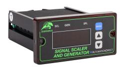
IronHorse signal conditioner, isolated, current or voltage input, current or voltage output, 120/240 VAC operating voltage, IP67, 1/8 DIN mount, screw terminals.
