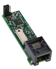
IronHorse GSD8 series communication module, ASCII, 1 port, (1) RS-232/RS-485 (RJ45) port(s). For use with IronHorse GSD8-240-5C-D and GSD8-240-10C-D DC drives.
