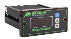
IronHorse GSD8 series DC digital drive, 120/240 VAC, 1-phase, 1/2hp at 90 VDC and 1hp at 180 VDC, 5A, NEMA 4X, 1/8 DIN mount, field-install reverse, high-speed pulse input, SCR output. Requires encoder.
