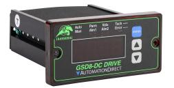
IronHorse GSD8 series DC digital drive, 120/240 VAC, 1-phase, 1/2hp at 90 VDC and 1hp at 180 VDC, 5A, NEMA 4X, 1/8 DIN mount, field-install reverse, high-speed pulse input, SCR output. Requires encoder.
