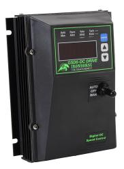
IronHorse GSD8 series DC digital drive, 120/240 VAC, 1-phase, 1hp at 90 VDC and 2hp at 180 VDC, 10A, RS-232/RS-485, ASCII, NEMA 4X, wall mount, field-install reverse, high-speed pulse or serial control input, SCR output. Requires encoder.
