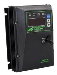
IronHorse GSD8 series DC digital drive, 120/240 VAC, 1-phase, 1hp at 90 VDC and 2hp at 180 VDC, 10A, NEMA 4X, wall mount, field-install reverse, current or potentiometer input, SCR and 4-20 mA control current output. Requires encoder.
