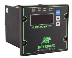
IronHorse GSD8 series DC digital drive, 120/240 VAC, 1-phase, 1hp at 90 VDC and 2hp at 180 VDC, 10A, NEMA 4X, 1/4 DIN mount, field-install reverse, high-speed pulse input, SCR output. Requires encoder.
