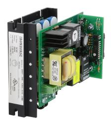
IronHorse GSD7 series DC reversing drive, 240 VAC, 1-phase, 1/25 to 1/4hp at 180 VDC, 1.2A, open frame, panel mount, built-in reverse, maximum 3 reverses/minute, potentiometer input, SCR output.
