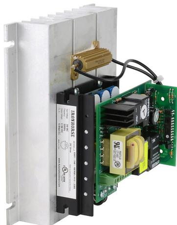
IronHorse GSD7 series DC reversing drive, 240 VAC, 1-phase, 1/4 to 2hp at 180 VDC, 10A, open frame, panel mount, built-in reverse, maximum 30 reverses/minute, potentiometer input, SCR output.
