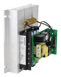
IronHorse GSD7 series DC reversing drive, 240 VAC, 1-phase, 1/4 to 2hp at 180 VDC, 10A, open frame, panel mount, built-in reverse, maximum 30 reverses/minute, potentiometer input, SCR output.
