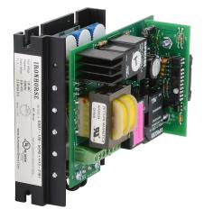
IronHorse GSD7 series DC reversing drive, 120 VAC, 1-phase, 1/8 to 1/2hp at 90 VDC, 5.5A, open frame, panel mount, built-in reverse, maximum 3 reverses/minute, potentiometer input, SCR output.
