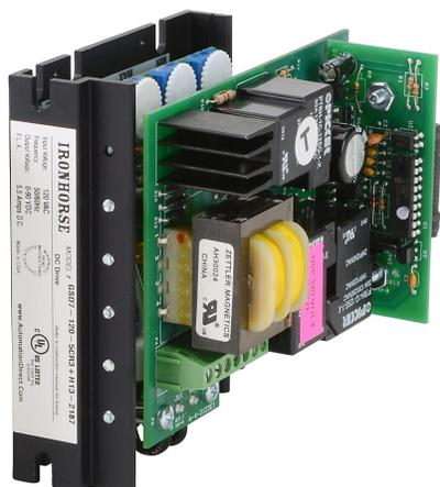
IronHorse GSD7 series DC reversing drive, 120 VAC, 1-phase, 1/8 to 1/2hp at 90 VDC, 5.5A, open frame, panel mount, built-in reverse, maximum 3 reverses/minute, potentiometer input, SCR output.
