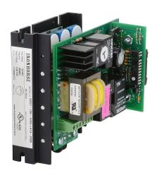
IronHorse GSD7 series DC reversing drive, 120 VAC, 1-phase, 1/15 to 1/8hp at 90 VDC, 1.2A, open frame, panel mount, built-in reverse, maximum 3 reverses/minute, potentiometer input, SCR output.
