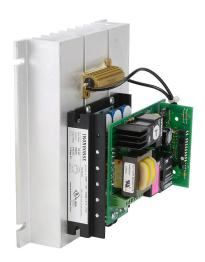
IronHorse GSD7 series DC reversing drive, 120 VAC, 1-phase, 1/15 to 1/8hp at 90 VDC, 1.2A, open frame, panel mount, built-in reverse, maximum 30 reverses/minute, potentiometer input, SCR output.
