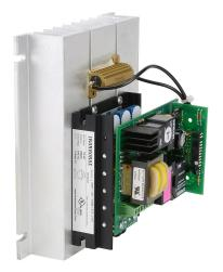
IronHorse GSD7 series DC reversing drive, 120 VAC, 1-phase, 1/15 to 1/8hp at 90 VDC, 1.2A, open frame, panel mount, built-in reverse, maximum 30 reverses/minute, potentiometer input, SCR output.
