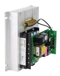
IronHorse GSD7 series DC reversing drive, 120 VAC, 1-phase, 1/8 to 1hp at 90 VDC, 10A, open frame, panel mount, built-in reverse, maximum 30 reverses/minute, potentiometer input, SCR output.
