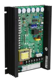
IronHorse GSD6 series DC full-featured drive, 120/240 VAC, 1-phase, 1/8 to 1-1/2hp at 90 VDC and 1/4 to 3hp at 180 VDC, 15A, open frame, panel mount, field-install reverse, potentiometer input, SCR output.
