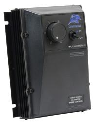
IronHorse GSD5 series DC general purpose drive, 120/240 VAC, 1-phase, 1/8 to 1hp at 90 VDC and 1/4 to 2hp at 180 VDC, 10.8A, NEMA 4/12, wall mount, field-install reverse, potentiometer input, SCR output.
