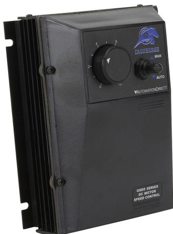
IronHorse GSD5 series DC general purpose drive, 120/240 VAC, 1-phase, 1/8 to 1hp at 90 VDC and 1/4 to 2hp at 180 VDC, 10.8A, NEMA 4/12, wall mount, field-install reverse, current, voltage or potentiometer input, SCR output.
